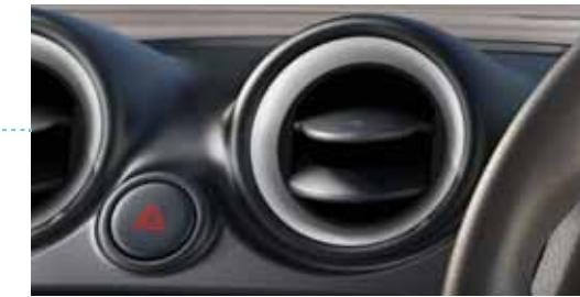
**4. 360° Air Vents for Surround A/C Ventilation:** Allows better control of airflow and air goes all around for your comfort.
